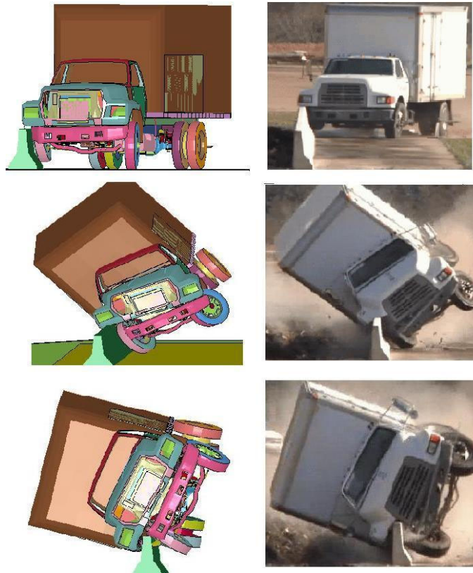
FIGURE 4 Left: Crash Performance Response of the FE Simulations Compared to the Full-Scale Crash Test (for update to NCHRP Test 4-12)
